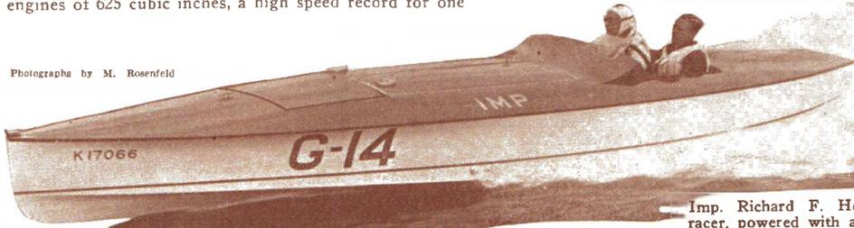
Imp, Richard F. Hoyt's Gold Cup racer, powered with a Wright marine engine established a record of 53.58 m.p.h. in the first heat
