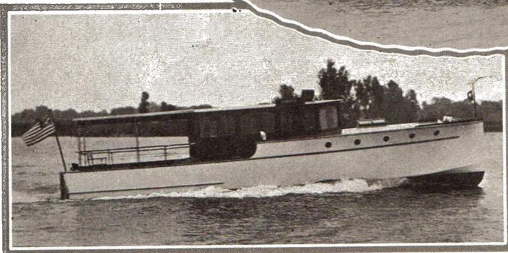
Nomabin is a 44 foot Vee bottom fast cruiser, also designed by Hacker-Fermann, and built for M. Whaling of Detroit. She is powered with a six cylinder Hall-Scott engine. A novelty is the auto type window lifts, fitted to all windows
