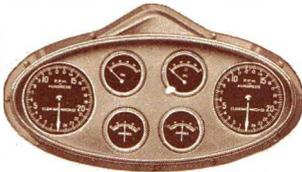
THE eighty-three foot express cruiser Rosewill, designed by Hacker & Fermann and built by the Defoe Boat & Motor Works, synchronizes its two 600 H. P. Packard engines with Elgin Chronometric Tachometers enclosed in the new Elgin Unit Control Board for twin-engined craft.
