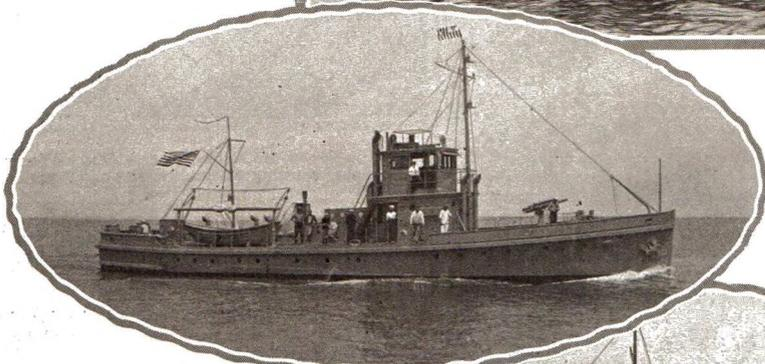
One of the thirteen 100 foot Coast Guard Cutters built by the Defoe Boat and Motor Works in quick time, last winter. These boats are powered with two 150 h.p. Winton Diesel engines. The hulls are heavily built of steel
