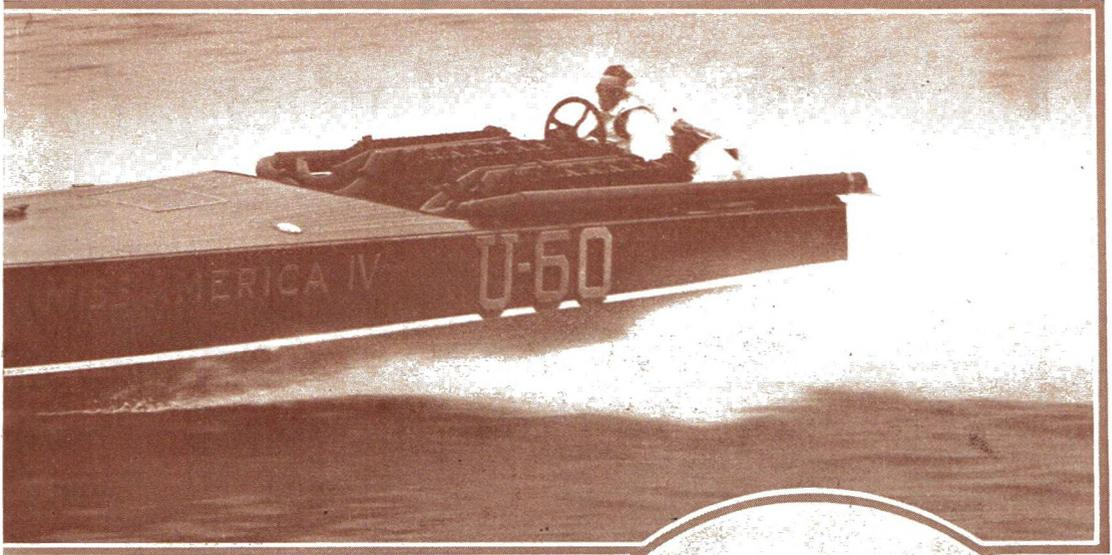
motors placed well aft in the hull. The shape of the underbody was slightly different, yet in all other ways the hulls and power plans were identical. Hyde wheels were used, Miss America III using one 20 x 40, Miss America IV, 21 x 38 and Miss America V, 21 x 37. Delco starting and ignition was used in all the boats.
